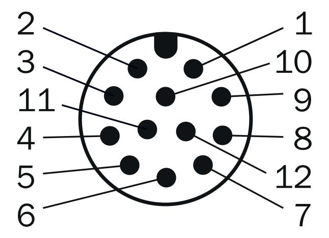
M12, 12-pin male connector, A-coded
