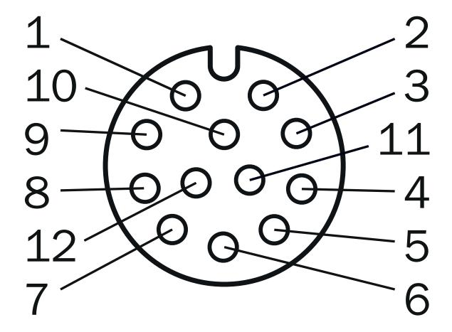
M12, 12-pin female connector, A-coded (I/O)
