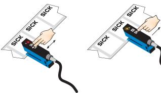
Press both the "+" and "-" buttons together, hold > 1 s and than release the teach-in buttons. The red LED flashes.
