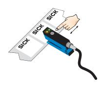
Release the teach-in button for < 20 s. If teach-in is successful, the function indicator (yellow LED) directly indicates the output state of the sensor. The switching t hreshold is now optimally set between carrier and label. The best possible operational safety is provided.
