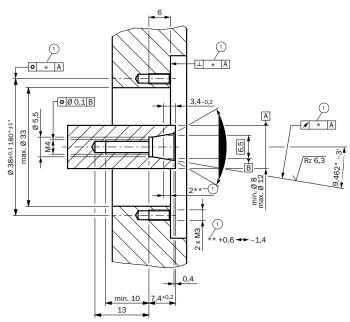
① The size of the tolerance reduces the permissible wave movement, see data sheet
