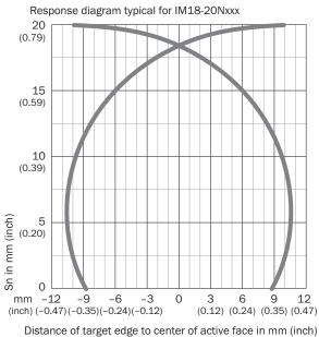
istance of target edge to center of active face in mm (inch) All dimensions in mm (inch)
