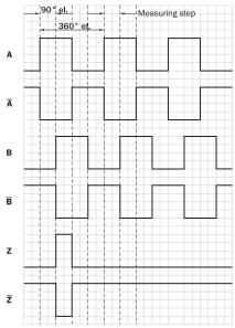
Cw with view on the encoder shaft in direction "A", compare dimensional drawing. 1 Interfaces G, P, R only for channels A, B, Z.
