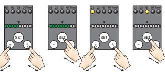
Position object in light field. Press SET button > 1 s. If requested adapt tolerance with "+" button (more coarse) or
